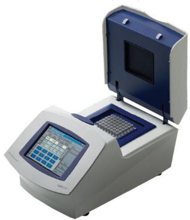
Polymerase Chain Reaction (PCR) is the process of replicating multiple copies of the genes of interest. The discovery of thermostable DNA polymerases, such as *Taq* Polymerase, has made it possible to manipulate DNA replication in the laboratory. It amplifies the quantities of DNA segments. Primers are used to identify the gene of interest and replicate them. These copies can then be separated and purified using gel electrophoresis.
